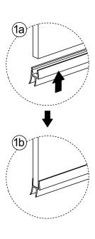
Ensure wall profiles are plumb. Adjust enclosure to be square and level. Wall post and profile should be adjust to square the doors and Ensure open door smooth.
